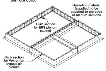
Anchor curb to roof deck structure in accordance with project construction documents.
